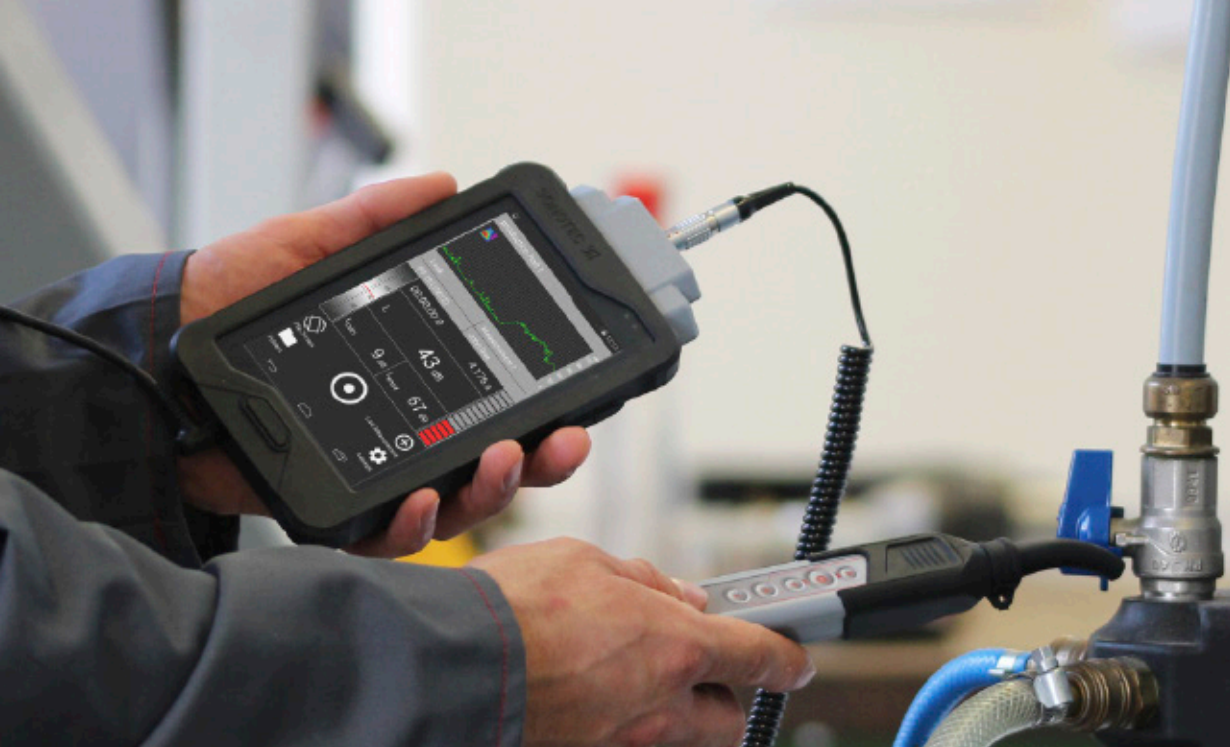
SONAPHONE Digital ultrasonic testing device for maintenance 4.0
