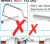
Don't use hacksaws to cut the pipe or leave burrs on the end of the pipe.
